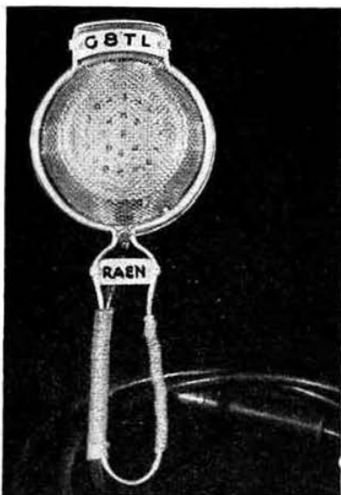
The neat housing for a Cosmocord Mic 6-4 crystal insert made from a sixpenny teastainer.
